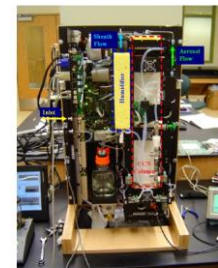
Cloud Condensation Nuclei Counter, US Patent 7,656,510
